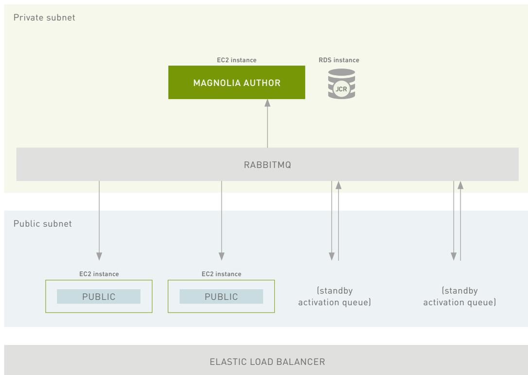
Using Amazon Web Services (AWS) and Magnolia CMS as an example, we offer four architectural blueprints for optimizing the deployment to ensure seamless integration. We discuss the advantages and disadvantages of each approach and offer recommendations to achieve autoscaling for high-performance and high-traffic scenarios.
